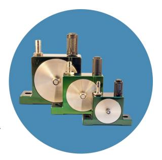
The Ball Vibrator VK is equipped with a ball, which rotates on ground raceways and generates high frequencies and fine amplitudes. The ball as well as the drop-forged and ground raceways are hardened to 62 HRC and attain very high running times as a result of the low wear. A dirty environment or slightly contaminated compressed air, however, does not have any effect on its functional operation. The VK can be operated in the vertical position with either oil-free or slightly oiled compressed air.
