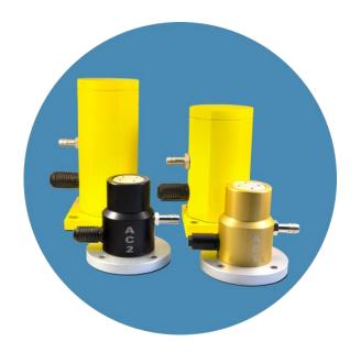
The Piston Vibrator AC generates very effective, linear amplifications and large momentum. The frequency is infinitely variable by regulating the pressure. This results in a broad spectrum of vibration. The AC has very compact installation dimensions and can be employed in all assembly positions. A dirty environment or slightly contaminated compressed air does not have any effect on its functional operation. The AC is maintenance-free and operates with slightly oiled compressed air.
